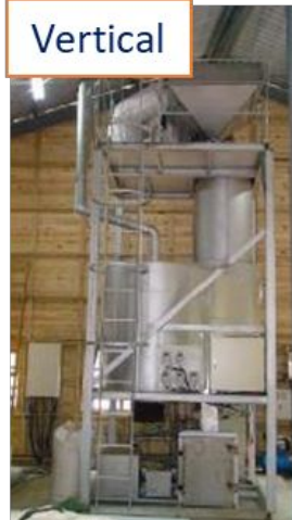
Continuous carbonization furnace
